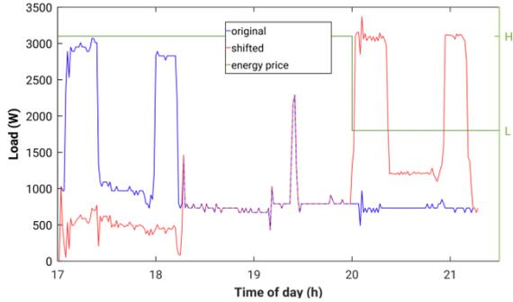
**Figure 2** Load shifting of individual appliances
