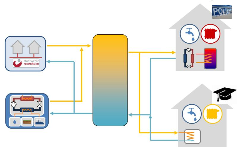
Heat for a low-temperature network is generated by a central heat pump supplied by environmental heat from a waste water stream. The close-by primary network return serves as back-up.
