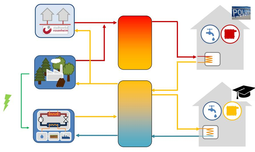
Heat for a high-temperature network is generated by a series connection of a central heat pump (first increase in temperature) with the two high temperature heat generation units combined heat and power and the primary network. The return of the high temperature network serves as flow for the low temperature network close by.
