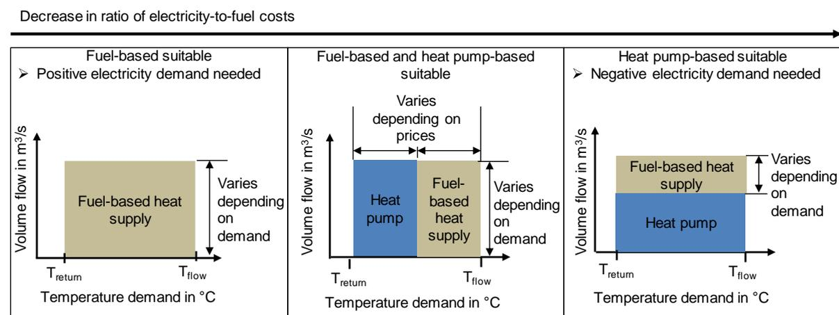
Figure 3: Interconnection of Heat pump and fuel-based boiler, depending on boundary conditions
