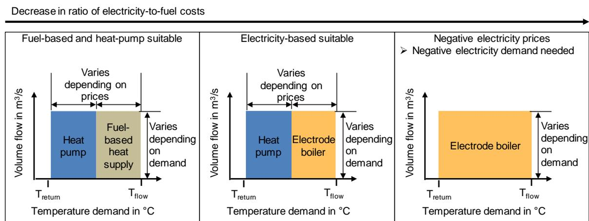
Figure 4: Interconnection of heat pump, fuel-based boiler and electrode boiler, depending on boundary conditions
